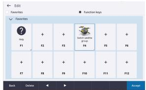
Now, unless you are actively in a measurement, tapping the assigned function will toggle between **ALL**, **SV set A**, **SV set B**
