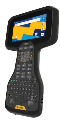
The Trimble TSC5 is the must-have controller for survey fieldwork and is fully integrated with Trimble's surveygrade instruments and software packages, including Trimble Access<sup>™</sup> Field Software and Trimble Siteworks Software. The TSC5 also supports the Trimble EMPOWER Module system, for use with the EM120 (Long Range Radio), EM100 (GNSS), and EM11X family (RFID/Barcode readers).
