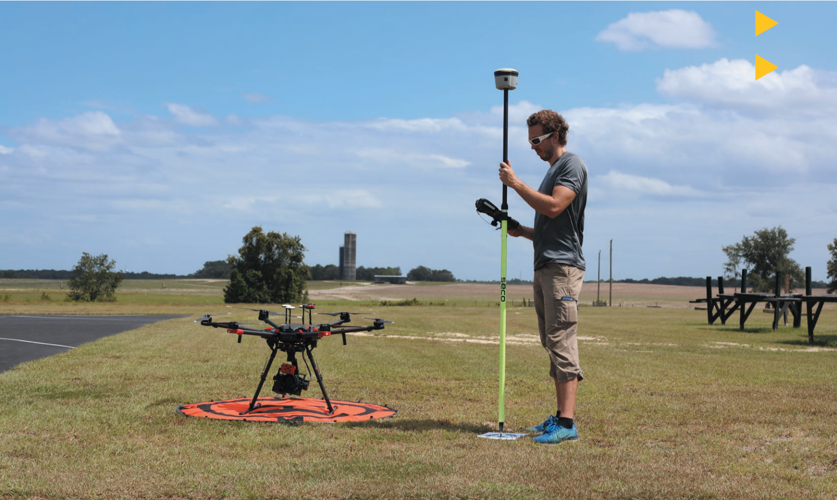
A technician uses Trimble GNSS to establish ground control prior to a UAV flight. Precise control for aerial imagery is essential for high-resolution crop assessment.
