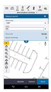
The TDC600 can connect to all supported GNSS receivers and most conventional instruments using Bluetooth. To perform a robotic survey you will need to connect the TDC600 to a TDL2.4 radio.
