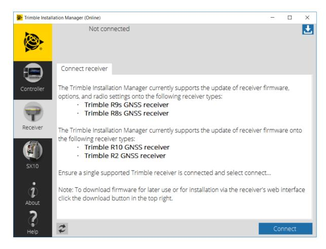
Trimble Installation Manager will display receiver-specific information. Select the firmware version you would like to install from the selection menu in the top right corner. Click on **Install** to start the installation process.
