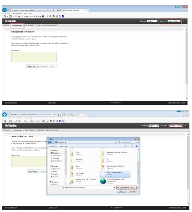
Step 14. If you have a job file with a calibration, linked files, feature code list, etc it can be converted to a template. Copy the "**Job File**" (.job) and paste it into the "**System Files**" folder.
